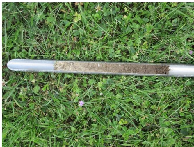
Figure 26: Soil profile within the soil sampler.
