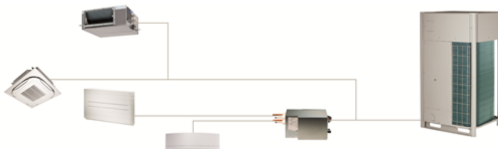
Figure 7-11: Example arrangement of multi-split equipment
